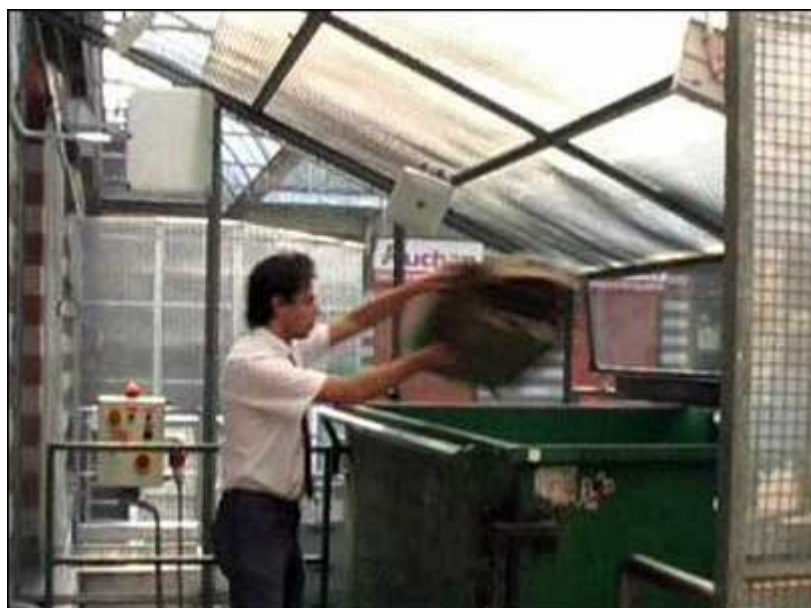
An RFID interrogator mounted above the trash compactor read the tags of empty cardboard cases.
